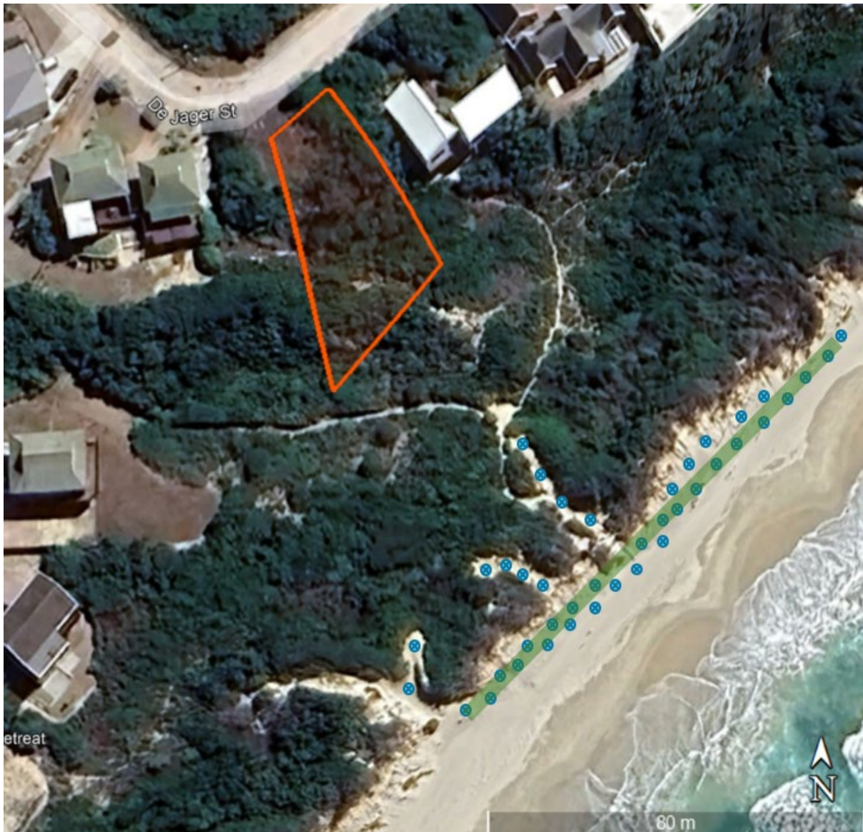
Figure 11: Interventions along the coast to trap sand with brushwood piles (blue circles) and establish pioneer dune vegetation (green highlight)
