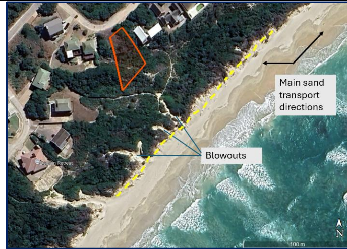
Satellite image showing Erf 1363 (orange outline) in relation to the steep eroding foredunes (yellow dashed line) and blowouts (van der Waal, 2026).
