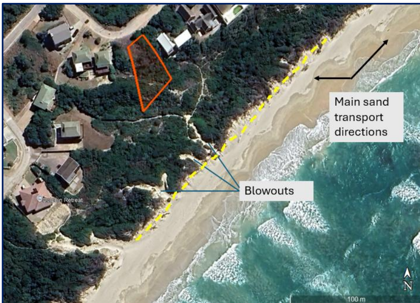
Figure 10: Satellite image showing Erf 1363 (orange outline) in relation to the steep eroding foredunes (yellow dashed line) and blowouts (van der Waal, 2026).
